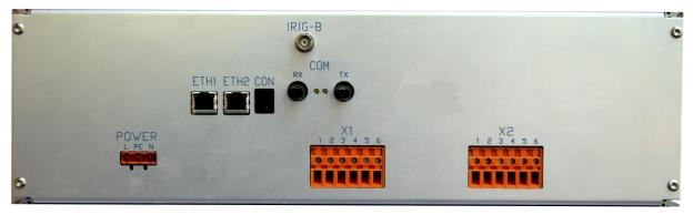
PMU is equipped with 6 analog inputs
