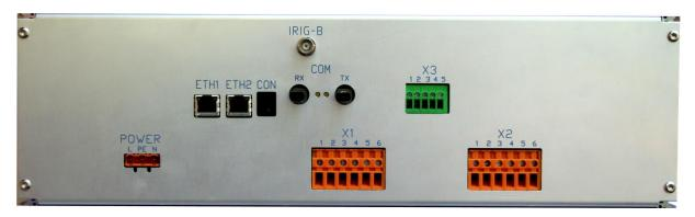
PMU is equipped with 6 analog inputs and 6 digital outputs
