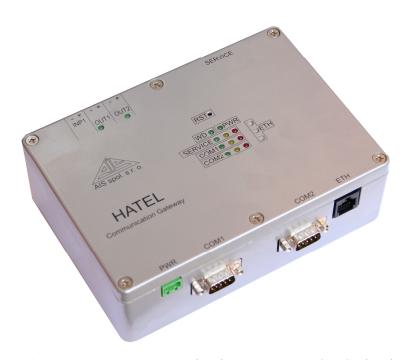
HATEL serves as communication gateway. The device is equipped with two serial channels, serial service port and ETHERNET channel 10/100Mbps.
